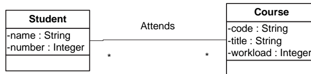
Fig. 15. Simple UML Diagram that shows a relationship between the students that attend courses
